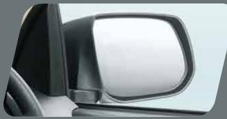
Large ORVM with casing Ensures no change in mirror position even after folding.
