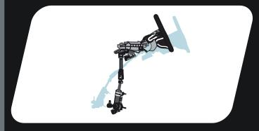
**Collapsible steering column** Added safety for the driver in the event of a frontal collision.
