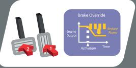
**Brake Override System** An intelligent system that reacts to panic braking of the vehicle, even when the accelerator is pressed with the brakes.
