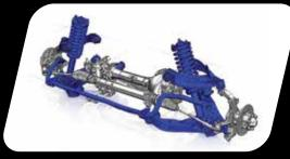
Front independent double wishbone suspension Heavy duty suspension for superior comfort and unmatched on-road durability.
