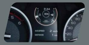
Multi-Information Display (MID) Advanced MID gives driver information about vehicle performance parameters. Odo meter, Speedometer, digital speed read out, instant mileage and average mileage, ambient temperature, elapsed time, current fuel range, DPD level indicator, AdBlue level indicator. Car like electroluminescent Instrument cluster
